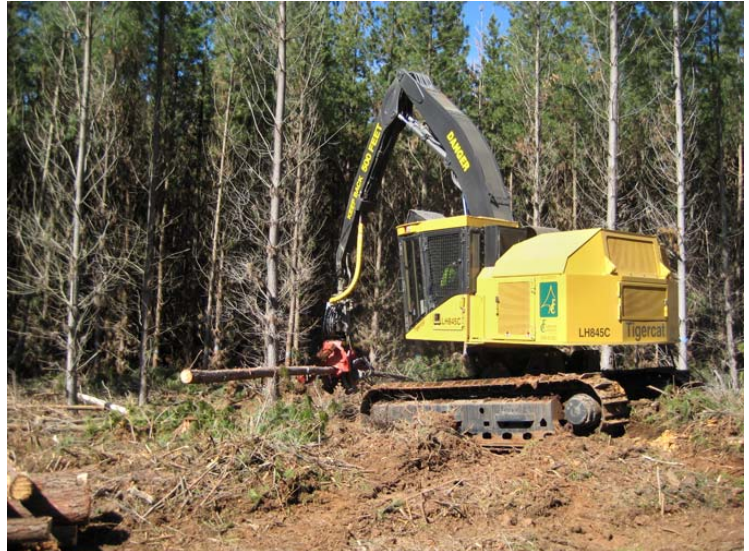
Tumut Valley Logging's new LH845C equipped with a Waratah 480 in thinnings
